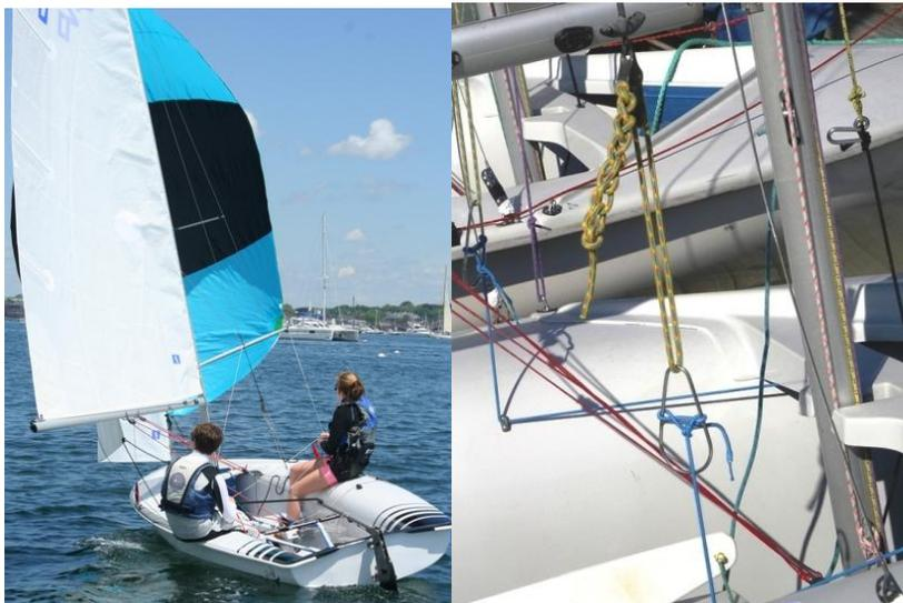
**Left: Usual crew positions when running under spinnaker. Right: The forward part of the crew's working area, with the trapeze wires held in place by shock cord led to the bails. The spinnaker is raised from and doused into a pouch just forward of the mast.**
